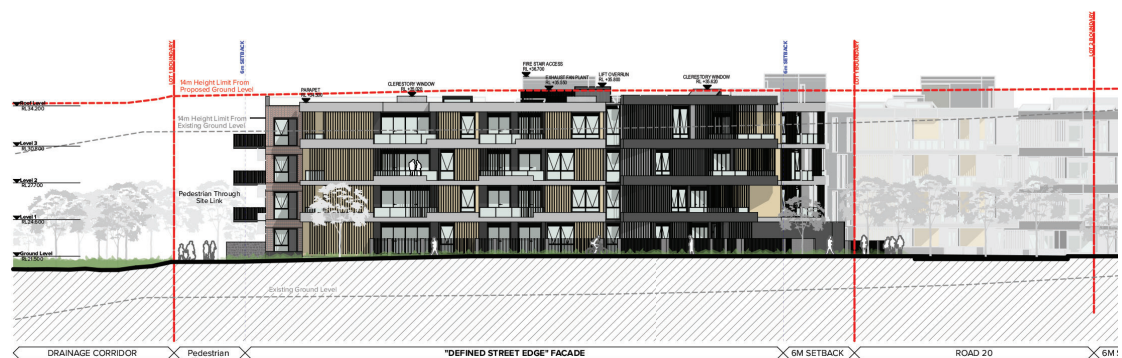
Sample extract of DA-820-003 elevations showing typical technical breaches of building heights.
